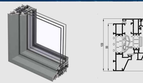
Slim Line 38 is a highly insulated system inward and outward opening windows and doors, which combines elegance and comfort, with a unique design. This special slender steel look is the perfect solution for modern architecture and renovation of steel-framed windows, respecting the original design but offering a thermally improved solution.
